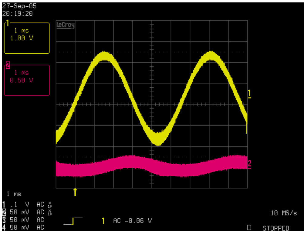
FIGURE 4. COMMON-MODE SIGNAL IMPROVEMENT FROM INPUT (YELLOW) AND OUTPUT (PINK)
